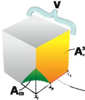
Grid generation for embedded boundary methods consists of computing areas, volumes, and moments associated with the intersection of each rectangular grid cell with the irregular domain.
