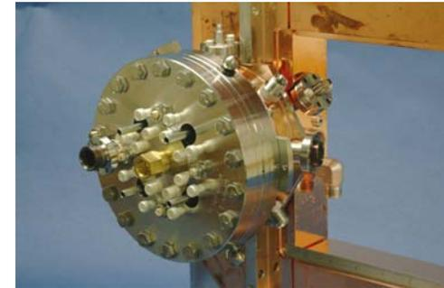
RF gun from SLAC (parallel simulation uses Zoltan)
