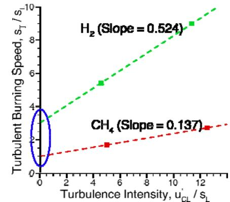
Quantifying dependence of burning rate on turbulence intensity for different fuels, with substantial impact on engineering design.
