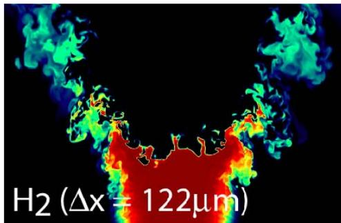
Adaptive mesh refinement calculation of Low Mach number combustion. Five levels of refinement, with the finest grid occupying 1/2% of the domain. Computed using 2400 processors on Cray XT4 at NERSC.
