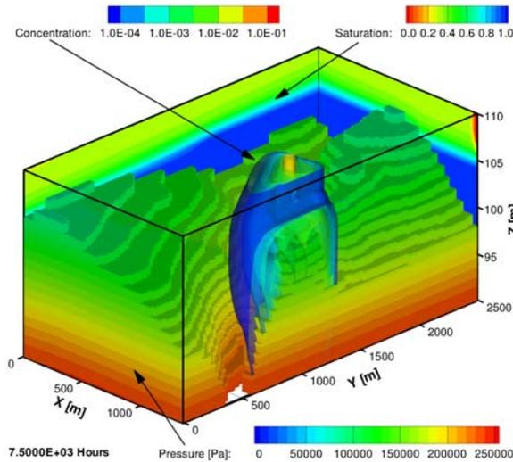
Sample computation using the PETSc powered PFLOWTRAN subsurface flow simulator and its parallel performance on the DOE leadership-class Cray XT3 system
