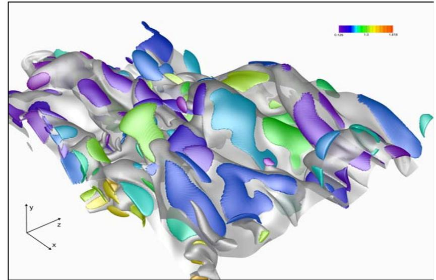
Topological Segmentation Allows Quantifying Turbulence From the Slope of Normalized Cumulative Distribution of Burning Cell Area
