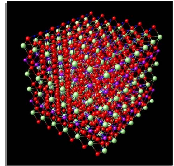
**Model of a  $\text{YBa}_2\text{Cu}_3\text{O}_7$
