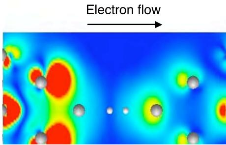
Shown at left is a single hydrogen molecule (in white) bridging palladium point contacts. At right, a density plot of the dominant transmitting electronic state reveals a significant reflection of charge at the left Pd contact, leading to a high resistance, consistent with recent experiments. (Red is high electronic density in the plot, blue is low.)
