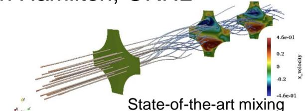
State-of-the-art mixing vane model resolved with CFD solver; used to optimized heat transfer in fuel rod bundles
