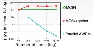
The parallel algorithm runs 300x faster than the sequential algorithm on 16K cores of NERSC/Cori.
