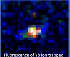
in High-Optical-Access ion trap
