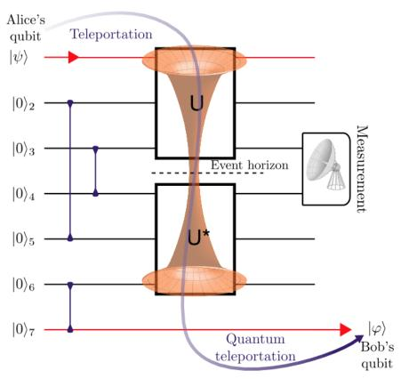
**Caption:** Schematic of the 7-qubit circuit, which uses quantum teleportation to detect information scrambling. The underlay depicts an analogy between our protocol and information propagation through a traversable wormhole.
