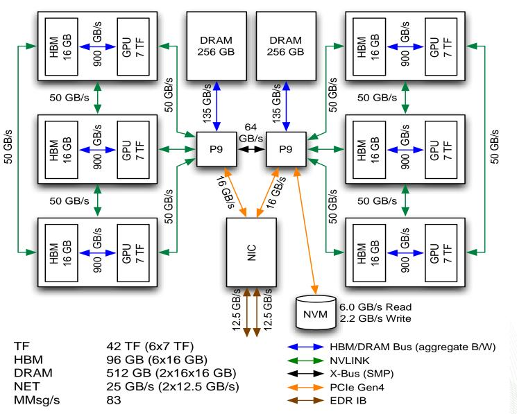
HBM & DRAM speeds are aggregate (Read+Write). All other speeds (X-Bus, NVLink, PCIe, IB) are bi-directional.
