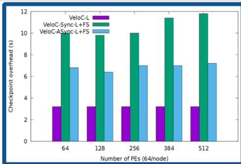
Preliminary experiments on Theta: Better scalability and performance for asynchronous vs synchronous mode
