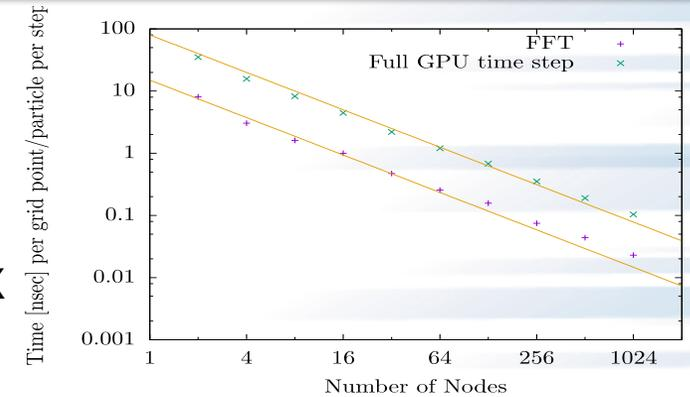
Weak scaling results for HACC on Summit Phase I up to 1024 nodes; straight lines represent ideal scaling. FFT optimization for Summit has not been carried out as yet.
