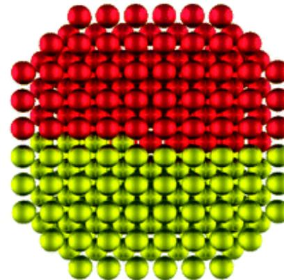
Alloy is stable if its energy is lower than the sum of the energies of the separated phases
