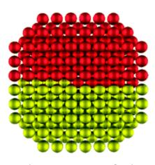
Alloy is stable if its energy is lower than the sum of the energies of the separated phases
