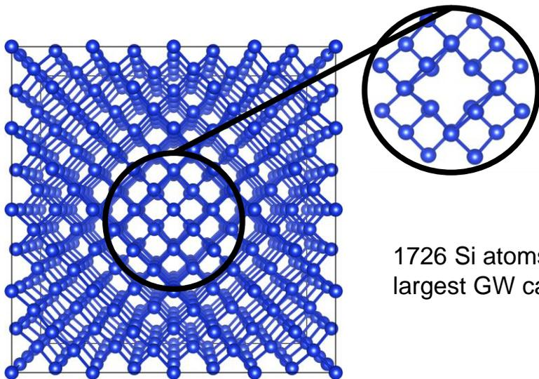
Schematic of di-vacancy defect and localized defect orbital in crystalline Silicon.
