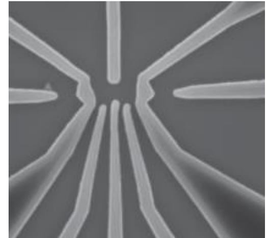
Electron micrograph of the fabricated silicon electrostatic electron-confinement chamber.
