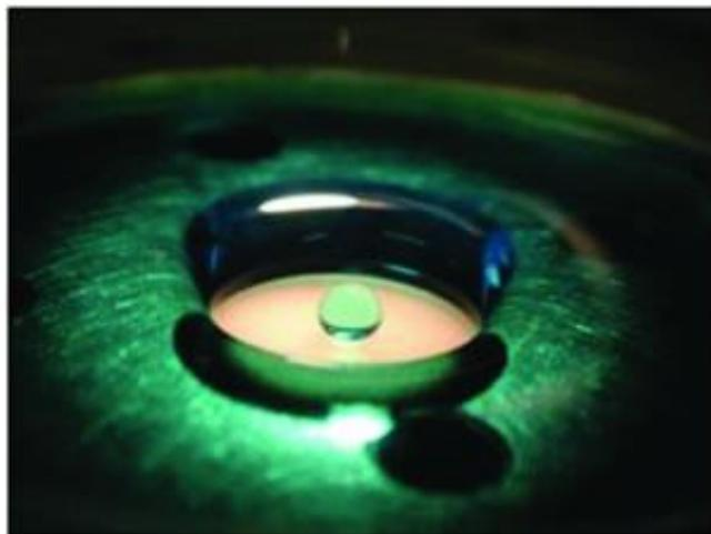
John Simpson, was able to change the wettability state by tailoring the surface topology and surface chemistry. The resulting structures consist of an outer layer of nanotextured sand with dimensions ranging from tens of nanometers to a few microns.
