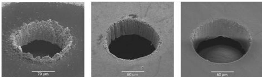
**Ultrafast, femtosecond pulse lasers (right) will eliminate machining defects in fuel injectors.**
