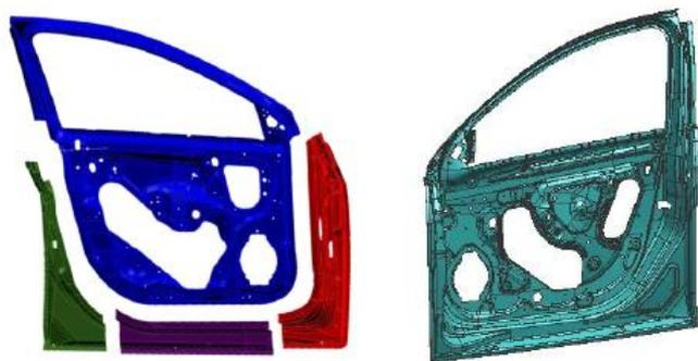
**Energy-efficient large thin-walled magnesium die casting, for 60% lighter car doors.**
