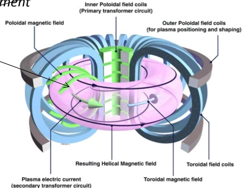
The **tokamak** is the leading magnetic confinement concept for fusion
