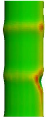
Cladding deformations and stress contour around MPS defect (displacements x20)
