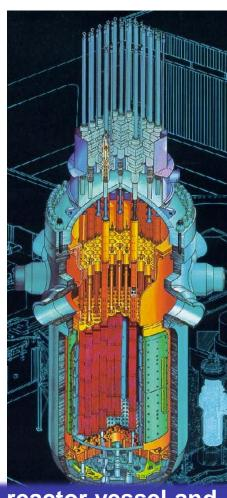
reactor vessel and internals
