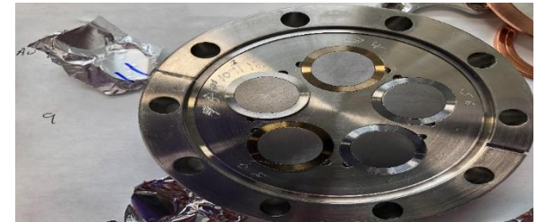
Preparation of parts for initial thermal bonding studies to inform next-gen LANL target design (top) all parts with various coatings (bottom) materials packaged for shipment for thermal pressing
