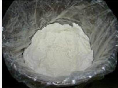
Initial processing of Li-7 at Y-12 completed FY 2016. Preparing for additional cleanup to meet product specifications for future molten salt reactors.
