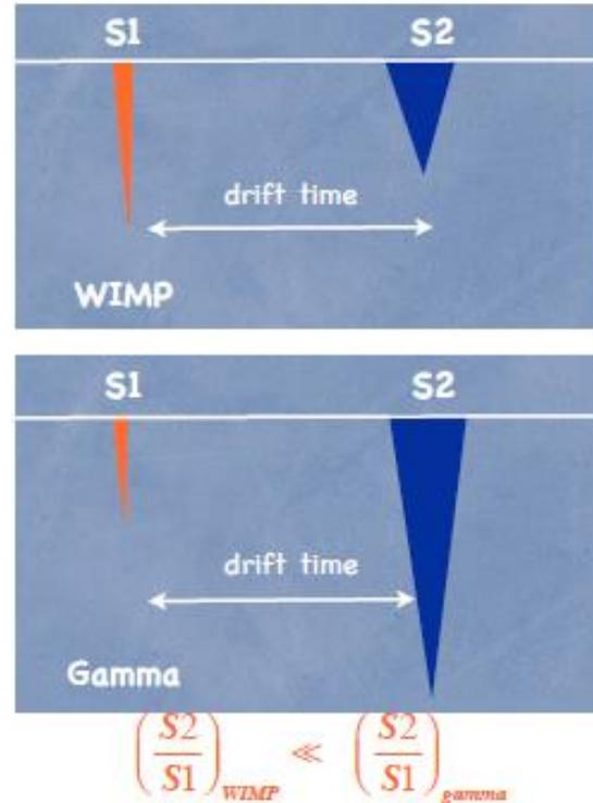
Prompt (S1) light signal after interaction; charge is drifted, extracted into gas phase and detected (S2)
