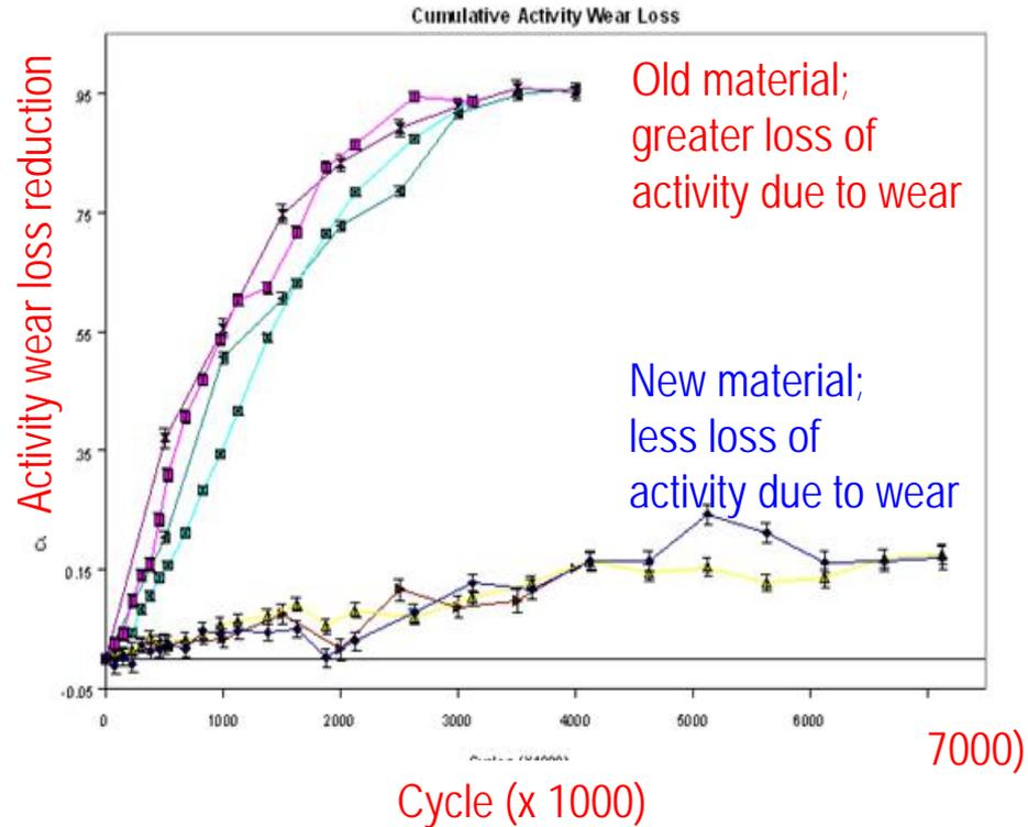
Cumulative  $^7\text{Be}$  activity wear loss versus wear cycles.
