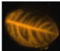
R3292 110mm diam. Hamamatsu PSPMT coupled to BC400 0.5mm thick plastic scintillator, 15 microns Mylar film and 25 micron Tedlar film were applied on top of the scintillating plastic. Detector ~600X more sensitive than dual planar PET.
