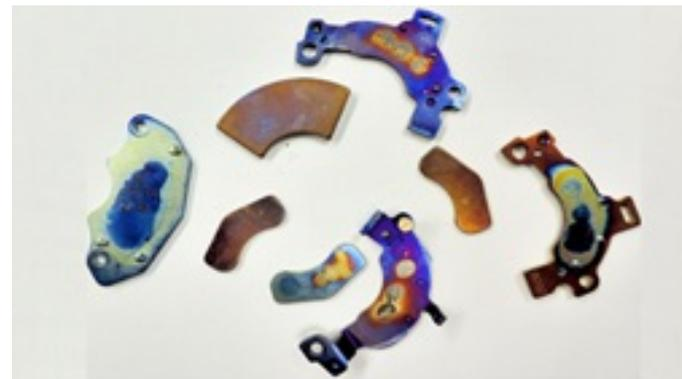
A photo of four voice coil magnets taken from a desktop or laptop computer and their brackets (which have mounting holes). These magnets are each about 10.5 - 15 grams, 1 - 1.25 inches long. These ones are colorful, because they have been overheated in the process of separation and demagnetization.
