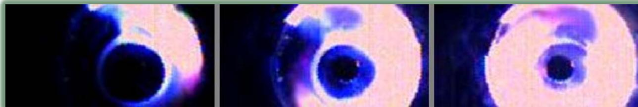
Consecutive frames from high speed camera (45000 frames per second) showing ~17000 rpm rotation of argon plasma.
