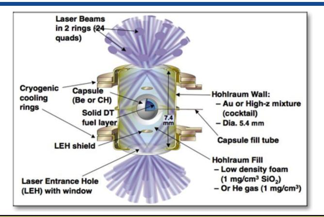
Fusion fuel implosion efficiency is 5-15% and the hohlraum temperature is about 10 keV
