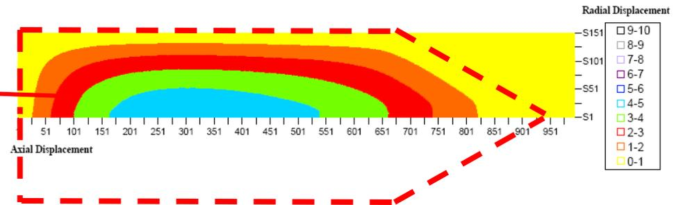
Potential buildup due to 50 million incident Cs ions per second in CPT gas catcher at 50 V/cm DC gradient.
