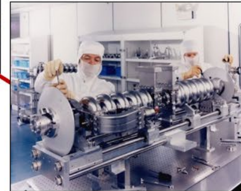
Superconducting Niobium radiofrequency cavities
