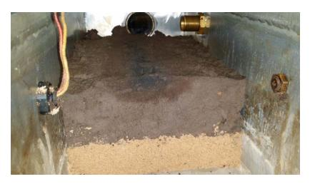
Figure 2-1 Decontamination cross section for a 10 MeV beam into a high-clay-content 5% contaminated soil [2-28].
