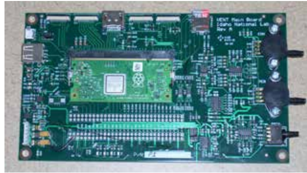
Fig. 5.60. Final prototype of the Idaho National Laboratory Wavetron computation, monitoring, and alarm board that replaced five printed circuit boards in legacy hardware. [Courtesy Idaho National Laboratory]
