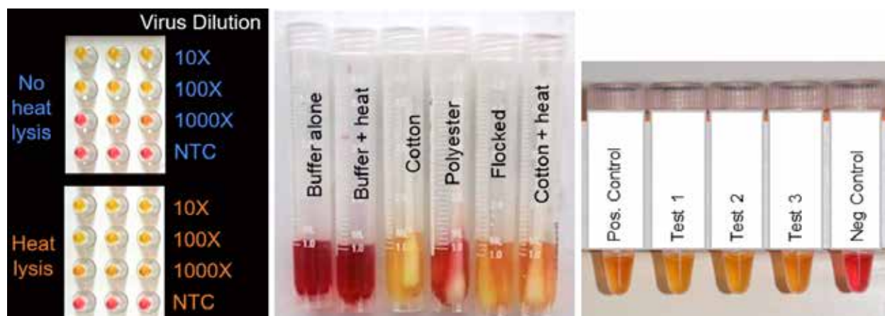
Fig. 2.32. Reveal-CoV test parameter development. A pre-amplification heat lysis/sample inactivation step improves colorimetric endpoint detection ~tenfold (left). Commercial swabs were evaluated to identify products with minimal effect on reaction color (center). A panel of five assays, including positive and negative controls and three virus-specific assays, were selected for optimal test performance (right). [Courtesy Lawrence Livermore National Laboratory]
