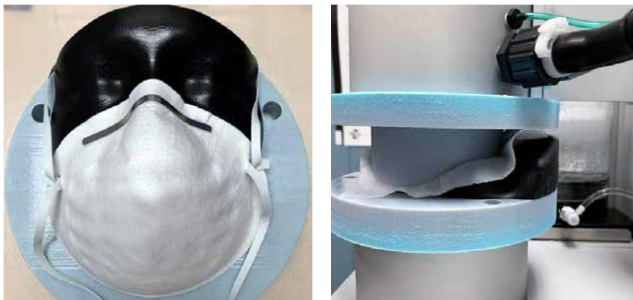
Fig. 5.26. Sandia National Laboratories human head test fixture for the ATI 100Xs automated filter tester. [Reprinted from Omana, M. A., et al. A Parameterization Study of Sew-EZ Materials: Types #6 and #8 . 2020. Sandia National Laboratories. DOI: 10.2172/1646968.]
