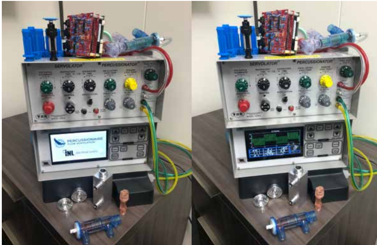
Fig. 5.61. Wavetron with prototype touch screen under Percussionaire VDR4 ventilator. Other components and molds shown. [Courtesy Idaho National Laboratory]
