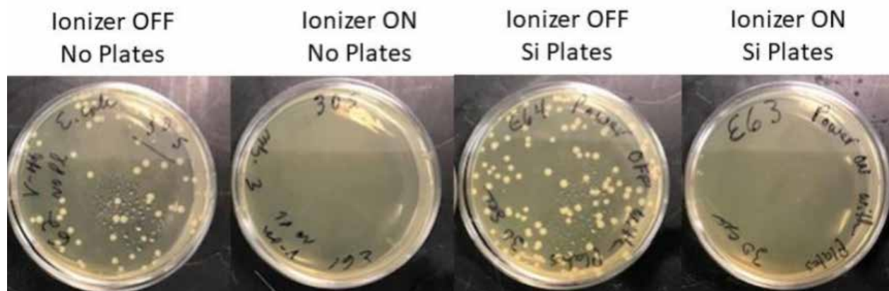
Fig. 5.31. E. coli colonies observed during tests of electrostatic precipitator. [Courtesy Savannah River National Laboratory]
