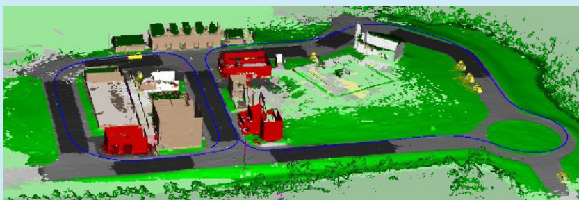
Figure 1. Computer vision techniques, such as semantic segmentation, enhance the capabilities of radiation detection measurements. A facility is segmented into distinct material classes. The trajectory of the vehicle carrying the computer vision sensors and the detectors is overlaid in blue [S85].
