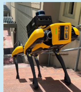
Figure 2. Boston Dynamics SPOT robot navigating stairs while carrying nuclear search equipment, including lidar and cameras [S86].
