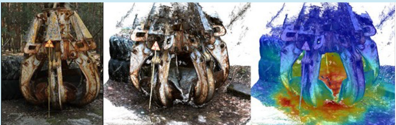
Figure 1. 3D reconstruction of a claw that was used to remove the radiologically contaminated debris from Reactor 4 of the Chernobyl Nuclear Power plant after the accident in April 1986. (left) A photograph shows the actual claw. (center) The photogrammetric reconstruction of the ~10 ft high claw with a simple radiation sign in front and some dumped truck tires in the back. (right) Visualization of the embedded cesium-137 contamination. This image was produced by projecting the gamma-ray image information onto the 3D photogrammetric surfaces. It illustrates that most of the cesium-137 contamination can now be found on the ground with dose levels of up to 0.4 mSv/h. The centimeter resolution reconstruction can be obtained within minutes [S83].
