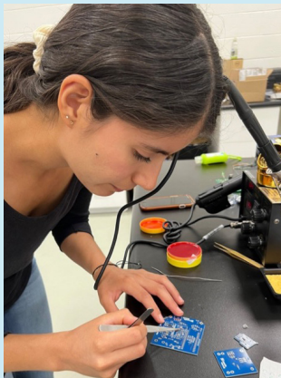
Diana Carrasco-Rojas solders a CosmicWatch detector for use at UTEP [S90].
